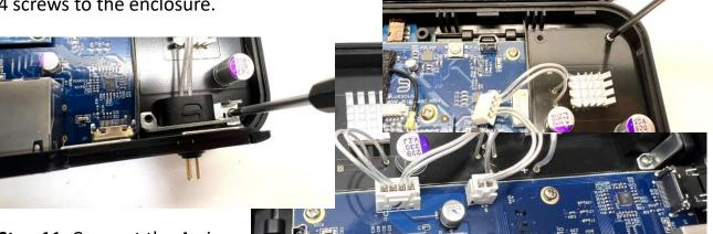
**Step 11:** Connect the 4-pin and 2-pin connectors in their matching sockets.
