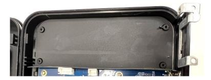
**Step 8:** Result after removing the internal SMPS and plastic cover sheet.
