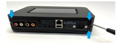
**Step 2:** Remove 3 screws to unlock the top of the Node.
