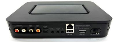
Now the Bluesound Node is ready to be connected to the Sbooster BOTW P&P ECO 5-6V.
