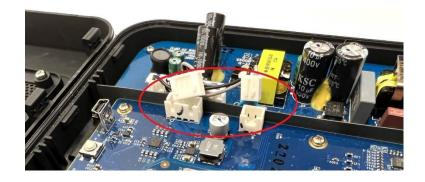
**Step 5:** Remove 4 screws of the Node's power supply board and take out the metal bracket that covered the connector.
