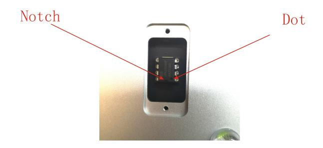
Make sure the notch and dot of the OPA2604 are on the same side with the notch of the socket.
