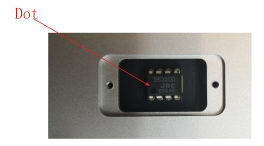
Make sure the dot of the NJM5532 are on the same side with the notch of the socket.
