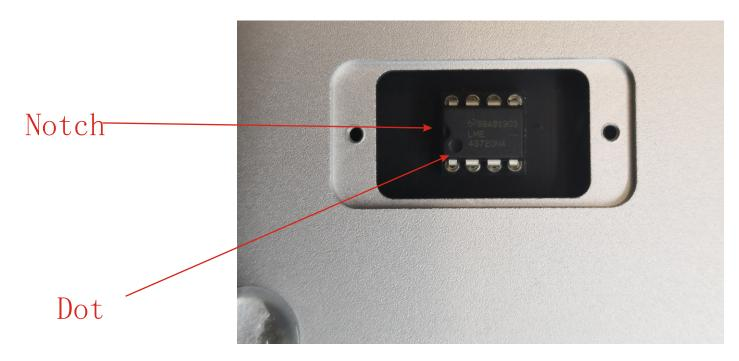
Make sure the notch and dot of the LME49720 are on the same side with the notch of the socket.
