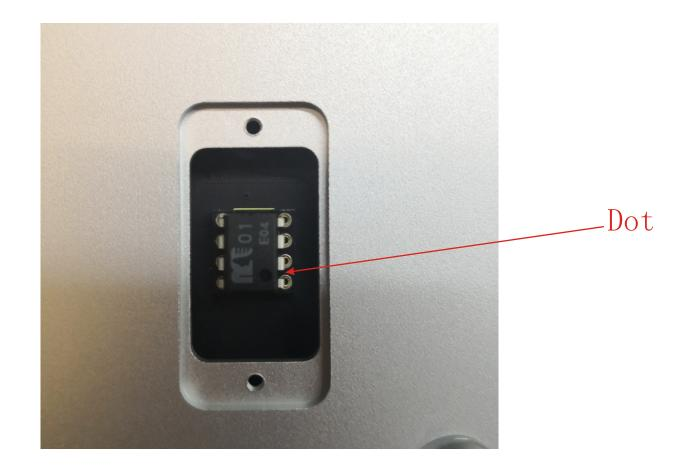
Make sure the dot of the MUSES01 are on the same side with the notch of the socket.
